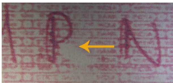
Fig. 4a-c. Discontinuity of background printing behind the letter “P” in 1 st , 2 nd and 3 rd generation photocopies produced by colour photocopier.
