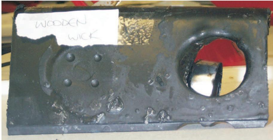
Fig. 4. Ferguson TV casing (after 37 minutes).
