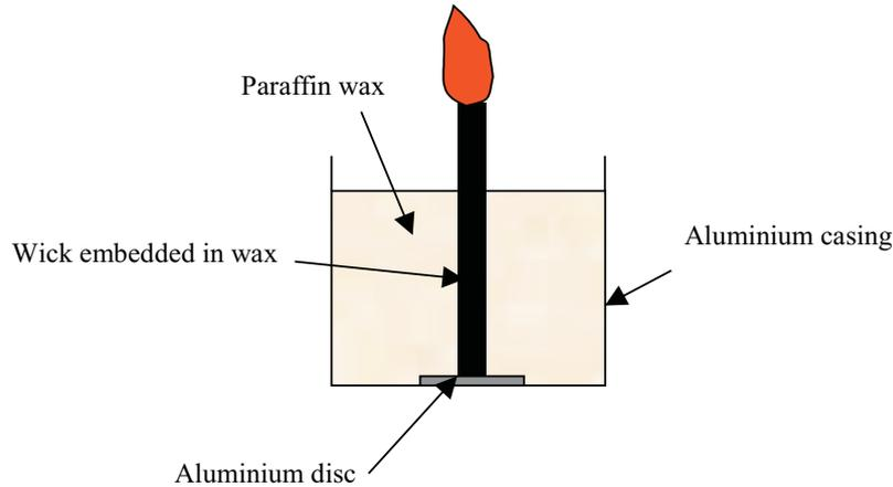
Fig. 1. Components of a typical night light.
