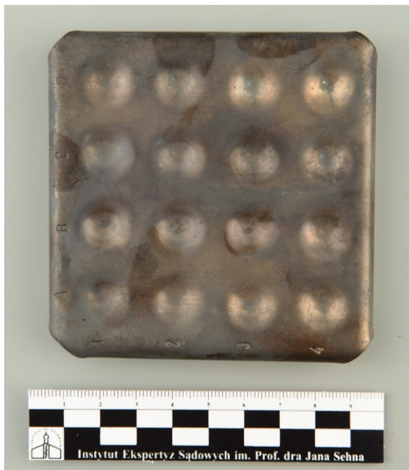
Fig. 2. An appearance of annealing holder used in Institute of Forensic Research (notation for glass fragments places: A, B, C, D – vertically positions; 1, 2, 3, 4 – horizontally positions).
